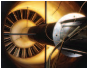
The NOTAR helicopter fan underwent testing in a custom test rig.
