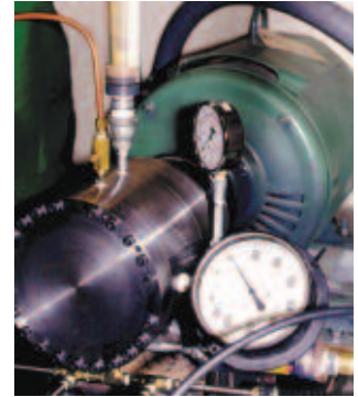
This custom test rig is for the development of advanced brush seals.
