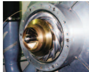
An industrial pump stage is prepared for performance and cavitation testing.
