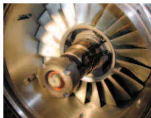
This axial compressor stage is instrumented with strain gauges and telemetry.
