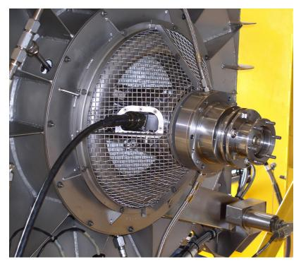
The VAROC High Precision Torque Measurement System (TMS) provides high speed torque measurement for turboshaft engine testing. It delivers accuracy, repeatability and reliability, and the system can be easily calibrated in the field.
