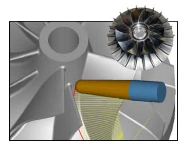
MAX-5 supports ruled blade surfaces with optional non-ruled edge constructions. It also includes options for roughing, plunge milling, hub finish, flank-milled blade finish, leading edge, fillet finish, and tip milling.
