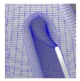
MAX-PAC can be applied to a wide range of turbomachinery components, including centrifugal and axial bladed parts. The software can scale components, rotate coordinate systems, and create many turbomachinery-specific design constructions as required. These can include leading- and trailing-edge shapes, constant and variable-radius fillets, and blade thinning. Splitter blades are also supported. The part model can be exported in IGES format ready for CAD systems.
