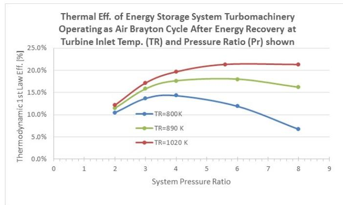
Fig. 7. Calculation of cycle efficiency for several turbine inlet temperatures,  $T_R$
