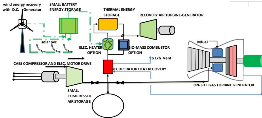
Fig. 1. Concepts NREC's "cross-over" system integrating a modular CAES with battery energy storage of power generated by renewable energy
