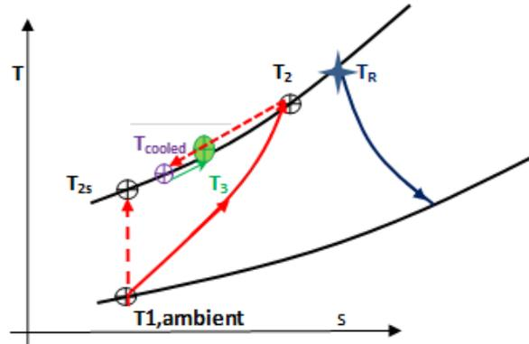
Fig. 3. Process path for air during Charging and Discharging sequence
