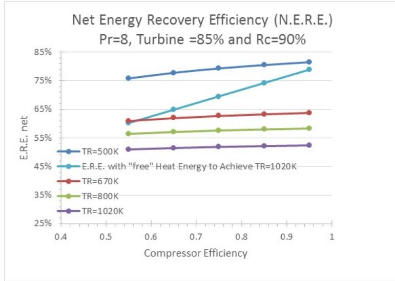
Fig. 5. Value of E.R.E. for an Rc=90% and turbine efficiency of 85%
