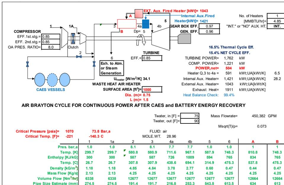
Fig. 9. Proposed Brayton Cycle engine as may be applied to "Cross-over" CAES-Battery Energy Storage
