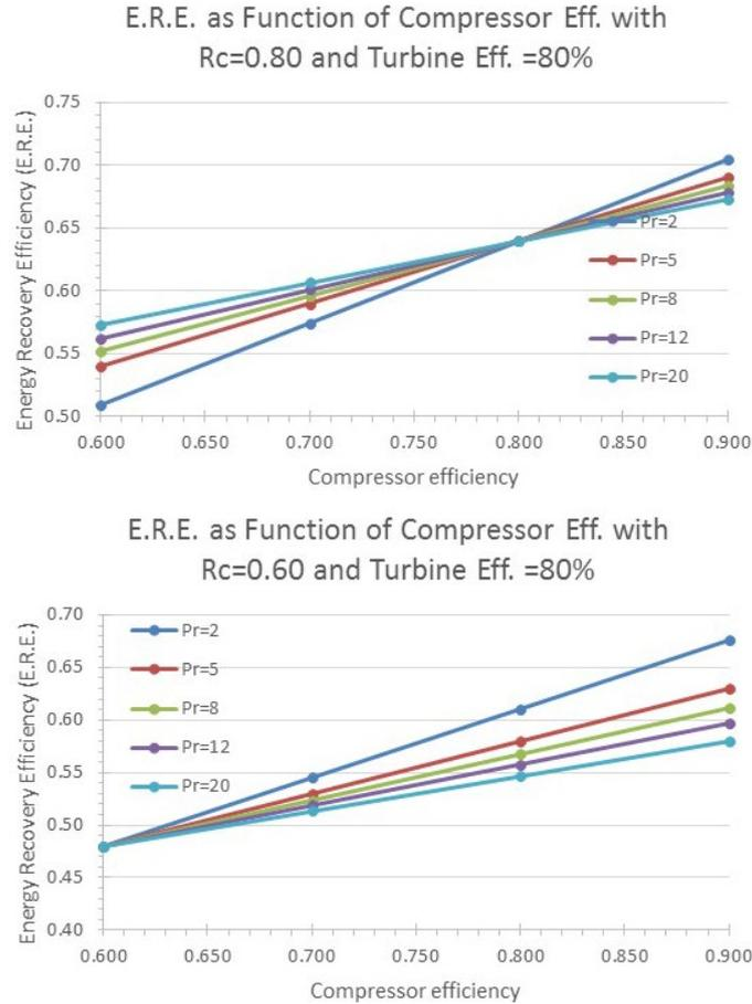
Figs. 4a-c. Results from a parameterization of the Energy Recovery Efficiency (E.R.E)
