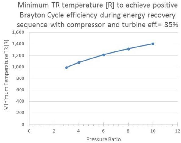
Fig. 6. Minimum temperature,  $T_{R,min}$
