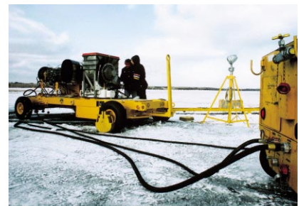
The VAROC is compact, lightweight, highly portable, and needs little support equipment, so it can be used anywhere regardless of climate.
