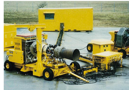
The U.S. Army incorporates state-of-the-art Concepts NREC air dynamometers in their mobile Flexible Engine Diagnostic/ test System (FEDS).
