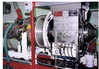
The VAROC-250 and the VAROC-35 can be used to test more than forty engine types covering a wide range of power and speed.
