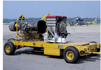
The VAROC Air Dynamometer is used worldwide by both military and commercial organizations to test a broad range of gas-turbine engines.
